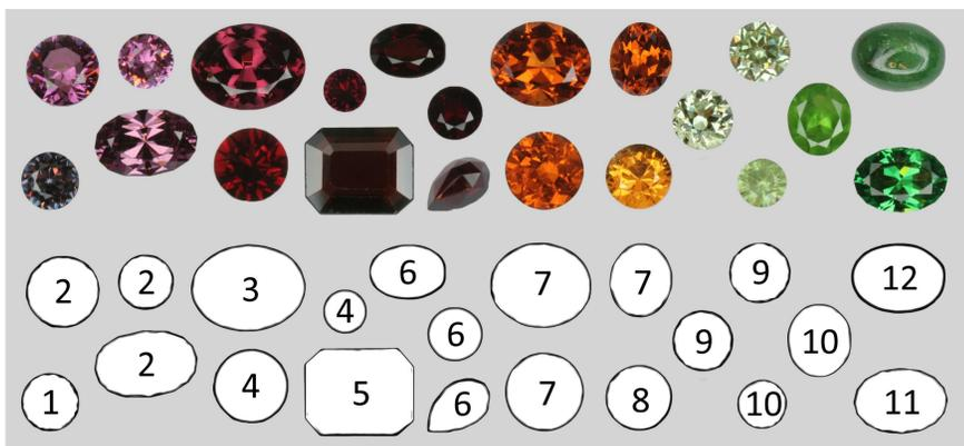
**Figure 1.** Range of color variation in garnet specimens. These samples are among those studied for this report: 1 – spessartine-pyrope; 2, 3, 4 – almandine-pyrope; 5 – grossular-andradite; 6 – pyrope; 7 – spessartine; 8 – spessartine-pyrope; 9 – grossular; 10 – andradite (demantoid); 11 – grossular (tsavorite); 12 – grossular.
